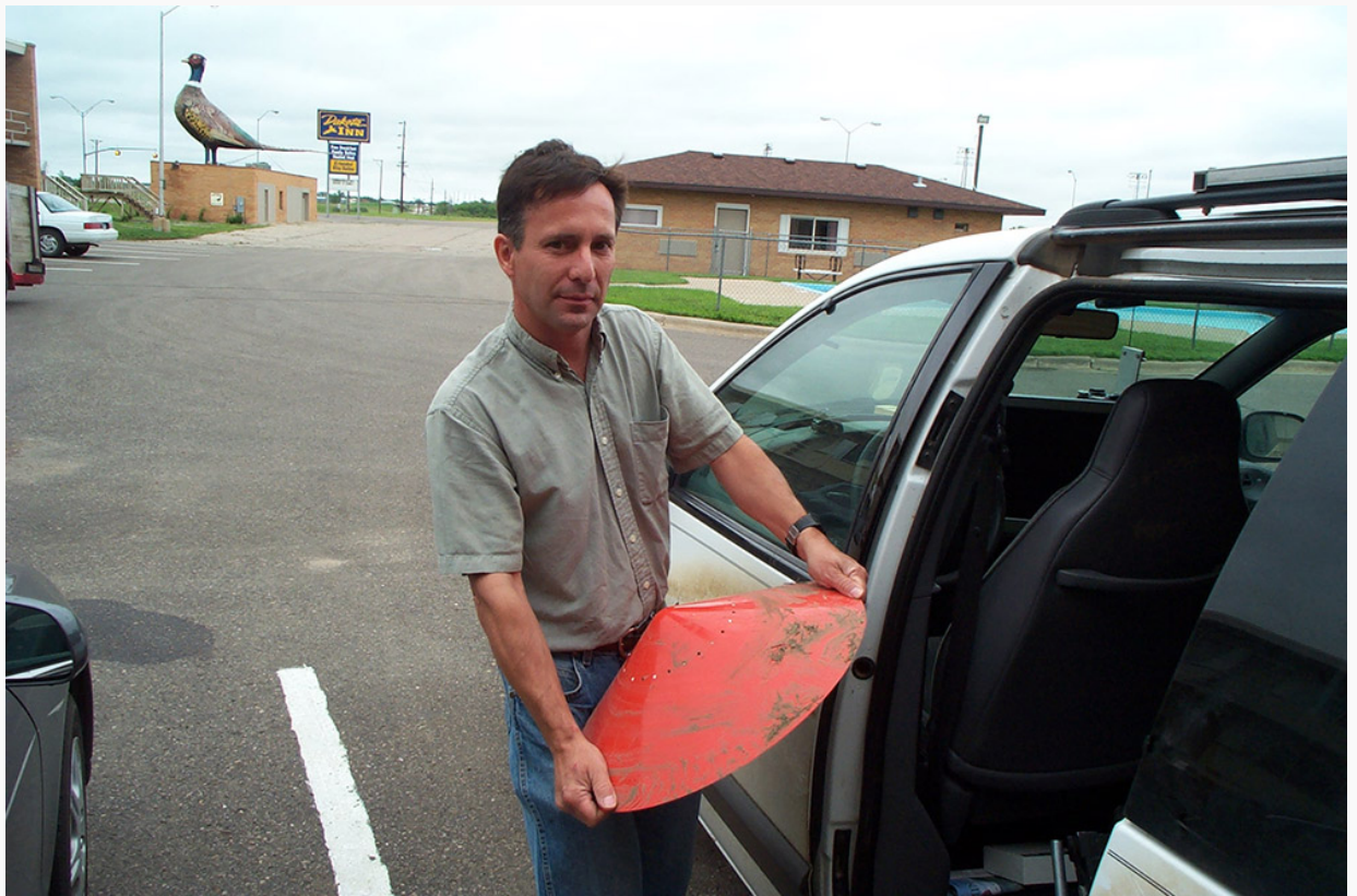
Tim Samaras holds one of the smaller probes he designed to set on the ground, right in the path of a tornado. It collects information on the intensity of the winds as the storm passes over it. Credit: T. Samaras
