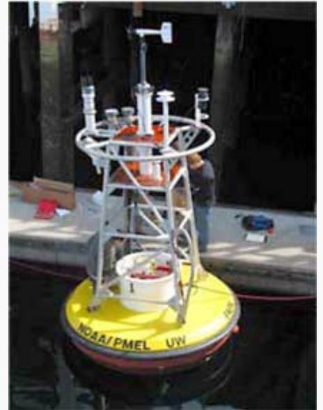
A buoy such as this one can carry equipment for directly measuring the pH of ocean water. Credit: NOAA
