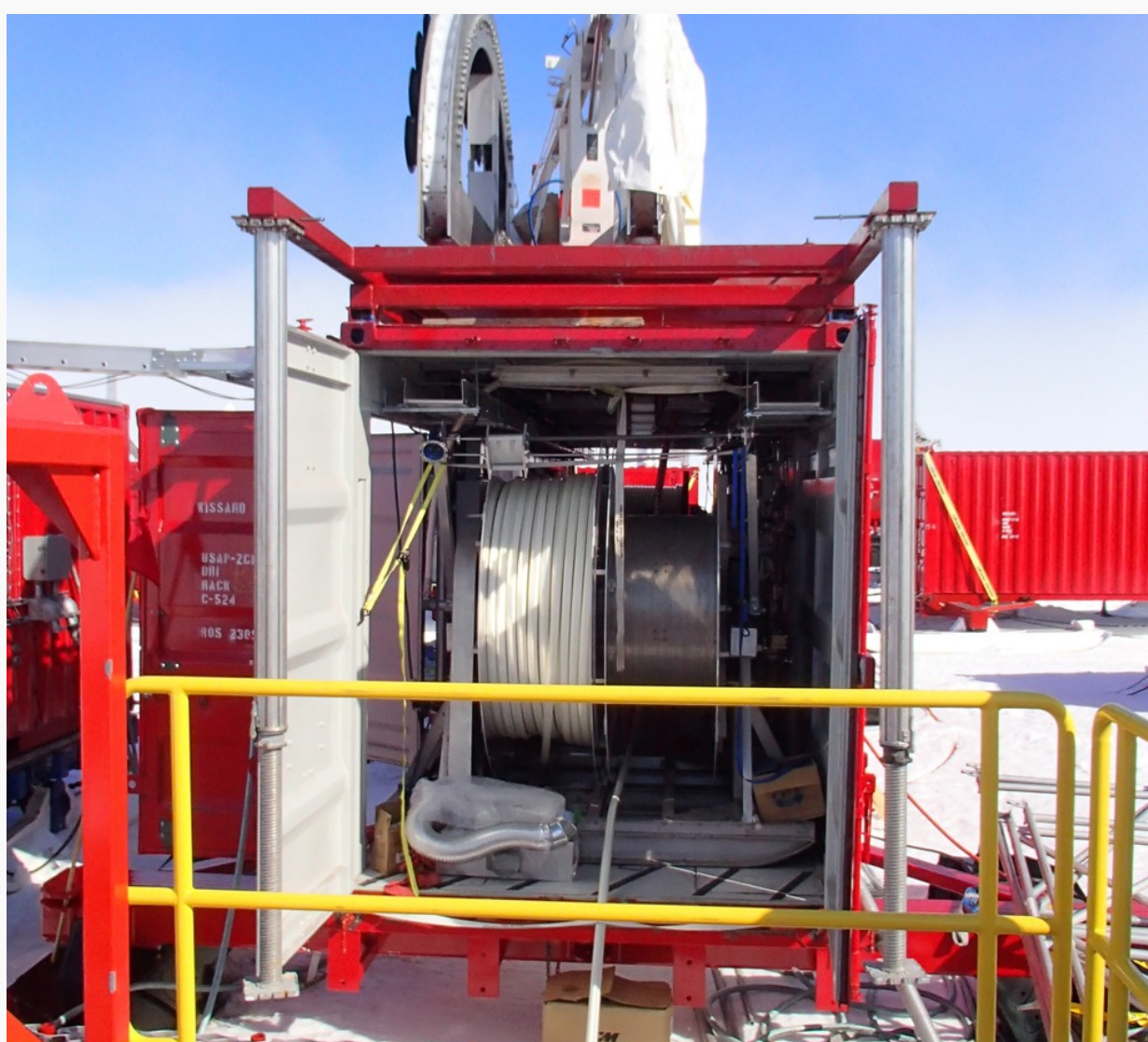
This 1,000-meter hose — spooled onto an enormous and very heavy container — was used as a drill to pierce deeply through Antarctica's ice. Credit: J. Raloff/Science News for Kids
