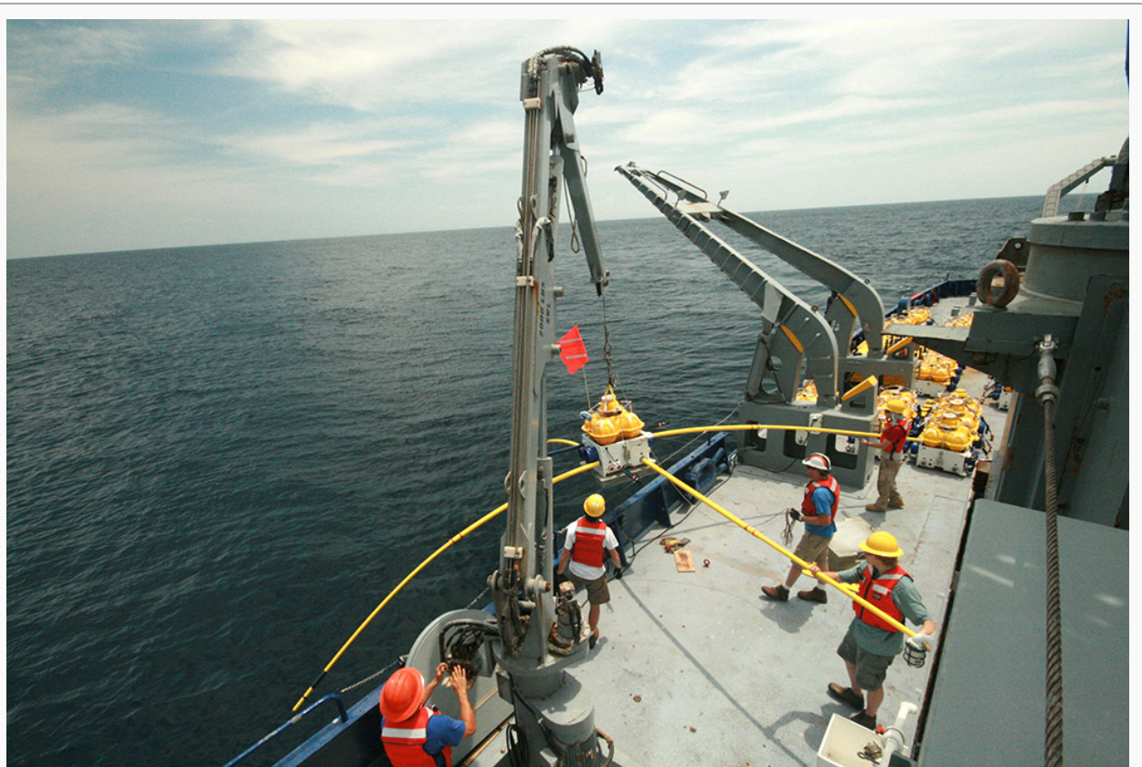
Scientists prepare to lower sensing equipment onto the Pacific Ocean floor. The equipment measured the seafloor rock’s ability to conduct electricity. They ran these tests at sites where one plate slides under another. Credit: Kerry Key, Scripps Institution of Oceanography at UC San Diego
