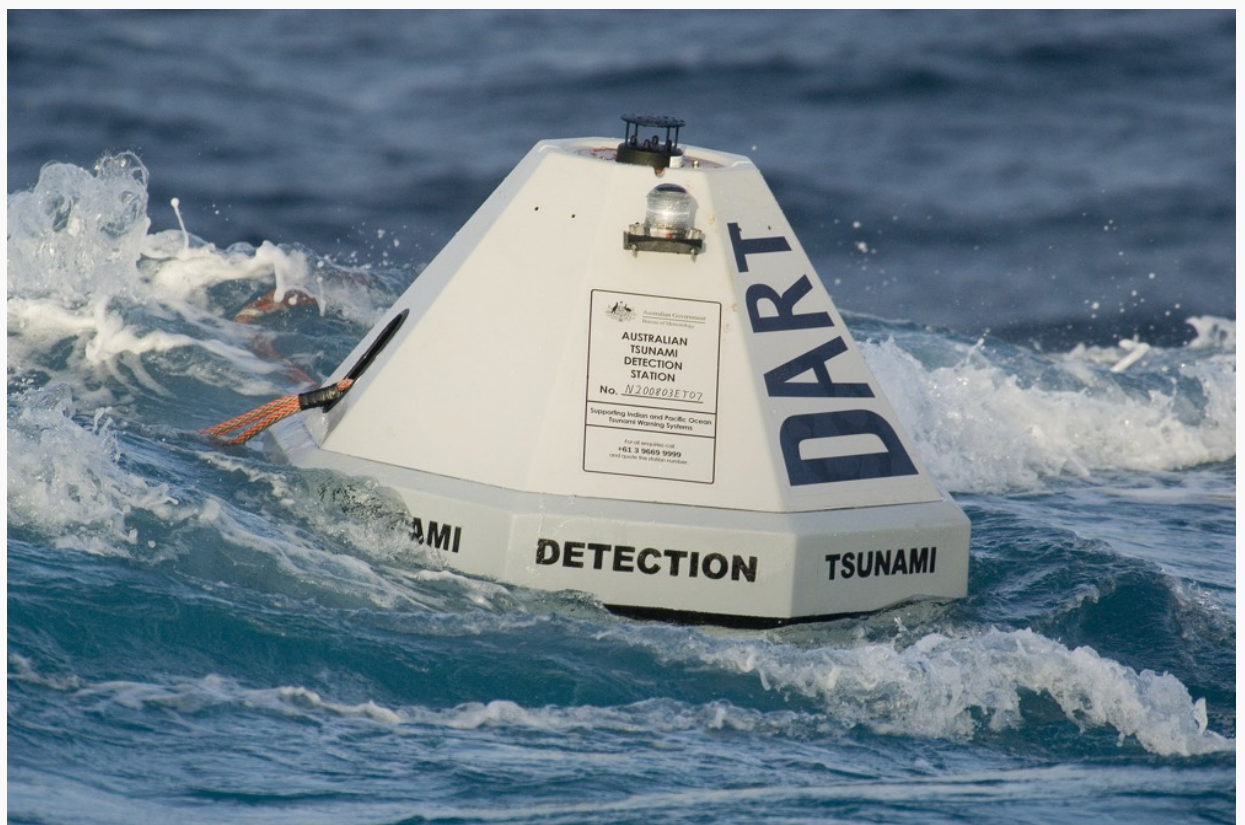
This buoy is part of the Deep-ocean Assessment and Reporting of Tsunami system. After an undersea earthquake strikes, buoys like this one record and transmit measurements of any tsunami waves. Credit: NOAA
